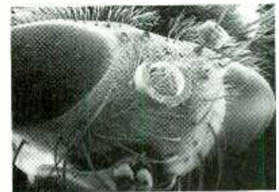
LASERLITH STATION (top) micro-machined these microminiature rings, shown adorning the head of a fly (bottom).
