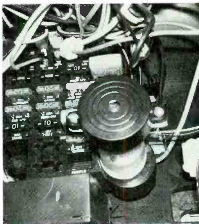
FIG. 7—THE STS FLASHER plugs into the original flasher socket.
