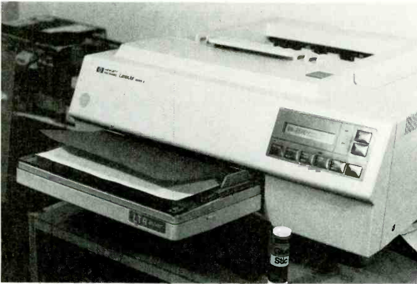
FIG. 3—IRON-ON TRANSFER FILM IS FED INTO THE LASER PRINTER. A backup sheet of paper can be attached to the leading edge of the film for support, if necessary.
