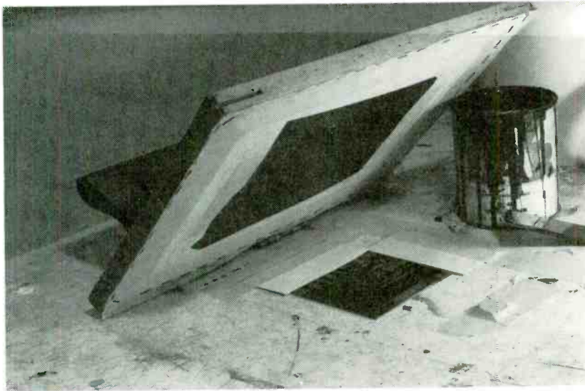
FIG. 8—PRINTED PC BOARD positioned beneath the screen image by the register guides.
