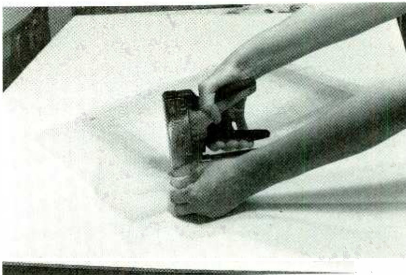
FIG. 2—THE FABRIC CAN BE STRETCHED and stapled to the frame by hand.
